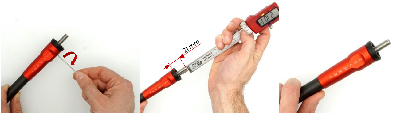
2.9 Lightly tighten the 2 mm clamping screw.
