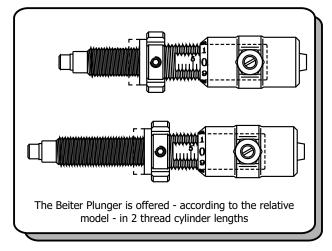
The thread cylinder is made out of high-grade refined steel, the springs out of stainless harmonic steel, the notching scale cylinder and the slotted nut out of anodised aluminum.
