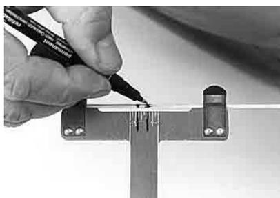
Set your nocking point with the checker and mark the correct position with a pencil.
