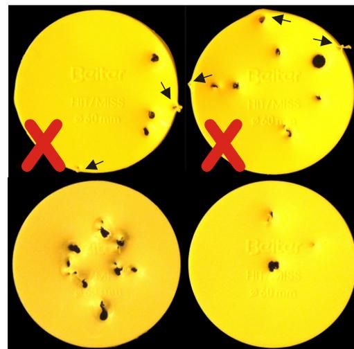
To extract Ø20mm Inserts hit by an arrow, it may be necessary to use a small hook (e.g. a crochet hook or a small hex wrench) Take care not to damage the hole's edge, which could cause the insert not to hold anymore. Therefore **DO NOT** use your fingers or the tool/hook as a lever.
