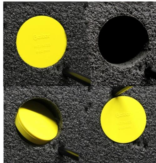
**ATTENTION! Do not** use the Hit-Miss Target System outdoors **under direct sun!** Due to different expansion between the foam and the plastic, the Inserts may not hold as desired!
