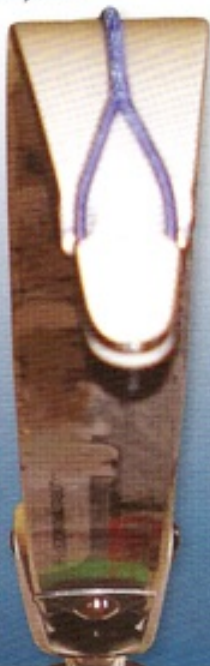
Limb tip off-centre requiring riser pocket adjustment
